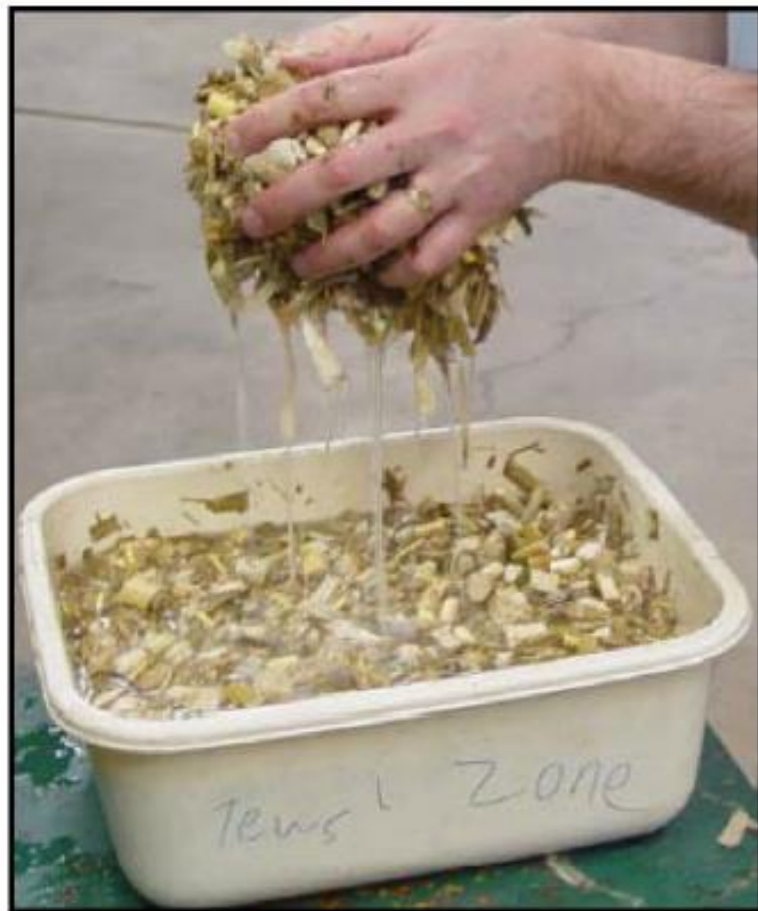
Figure 3. Skimming and removing the floating stover.
